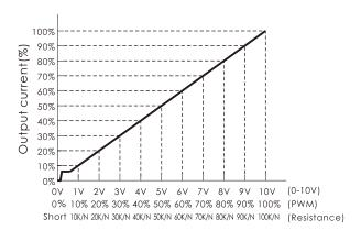
● 10V PWM signal for output current adjustment(typ.): frequency range:100Hz~3KHz
