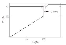
In the constant current region, the highest voltage at the output of the driver depends on the configuration of the systems.
