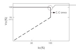
In the constant current region, the highest voltage at the output of the driver depends on the configuration of the systems.
